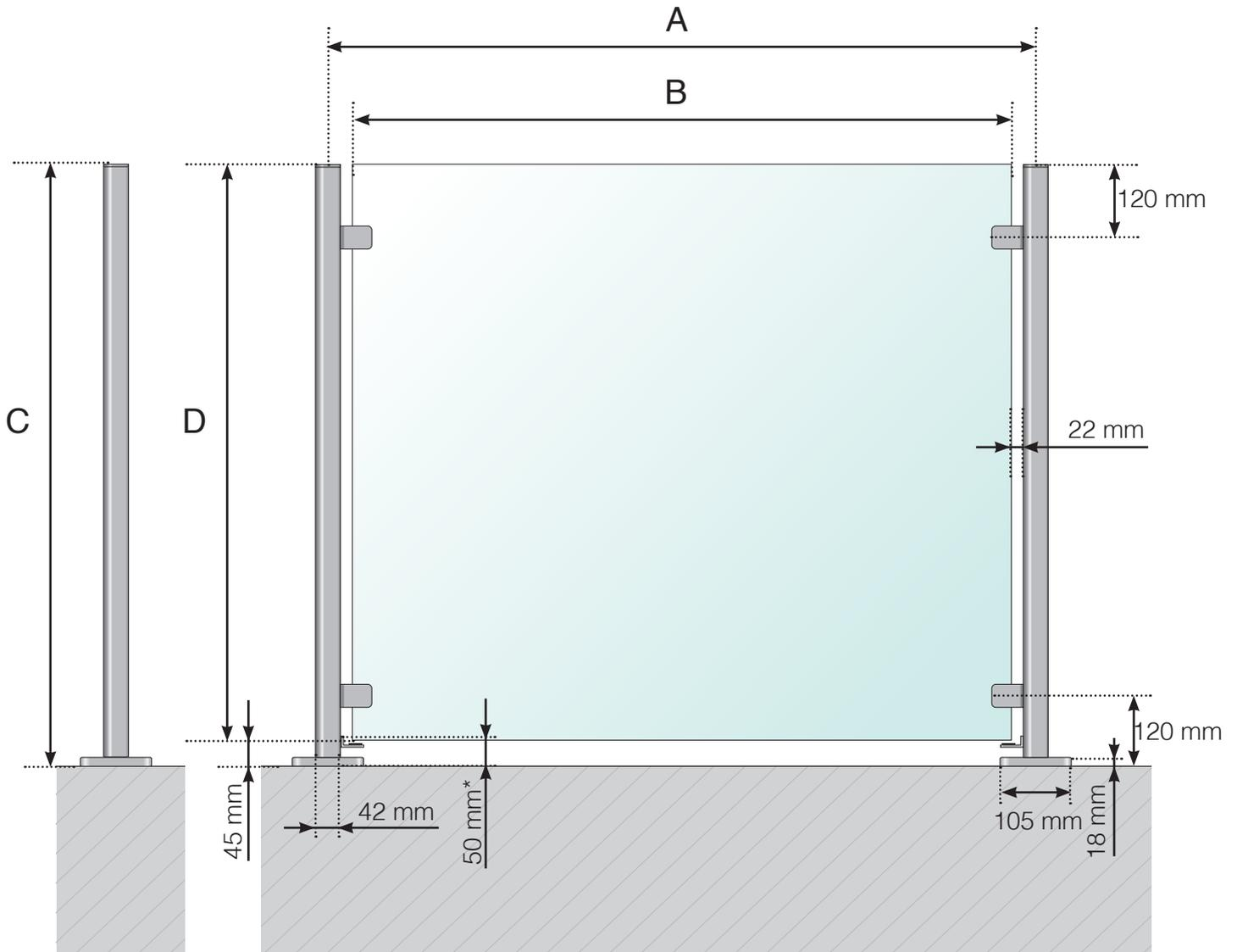
A - The c/c dimensions of the posts depend on the length of the sides and number of sections
